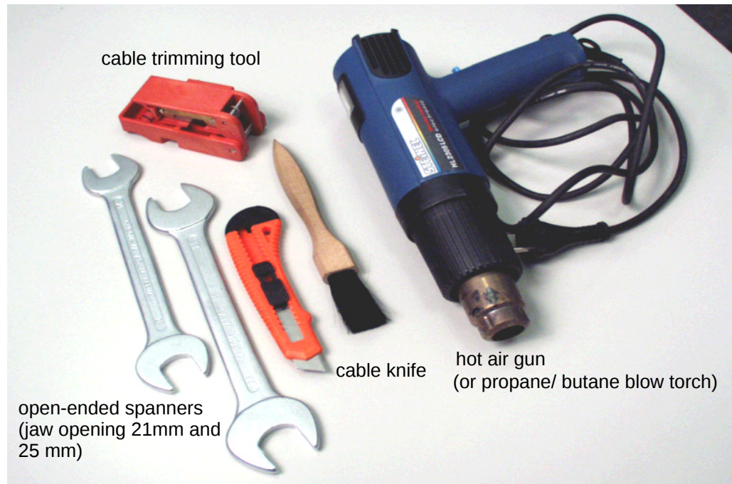
Fig. 2.44 Tools for jumper fabrication
