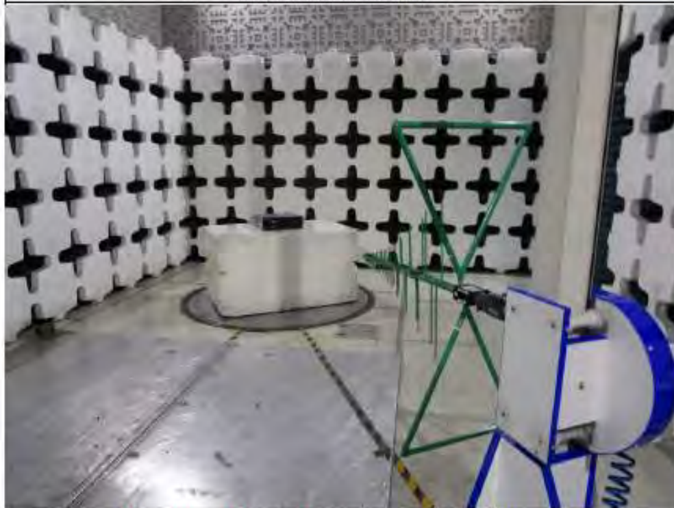
Test Setup for Spurious Radiated Emissions, 30MHz – 1GHz – Antenna Polarization Vertical
