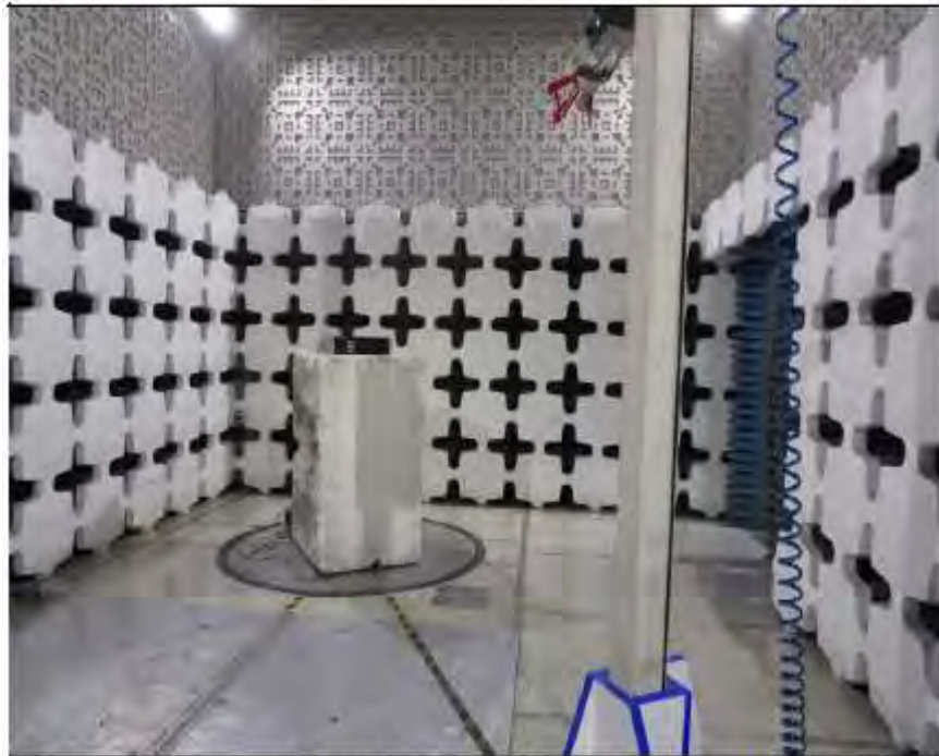
Test Setup for Spurious Radiated Emissions, Above 1GHz – Antenna Polarization Horizontal
