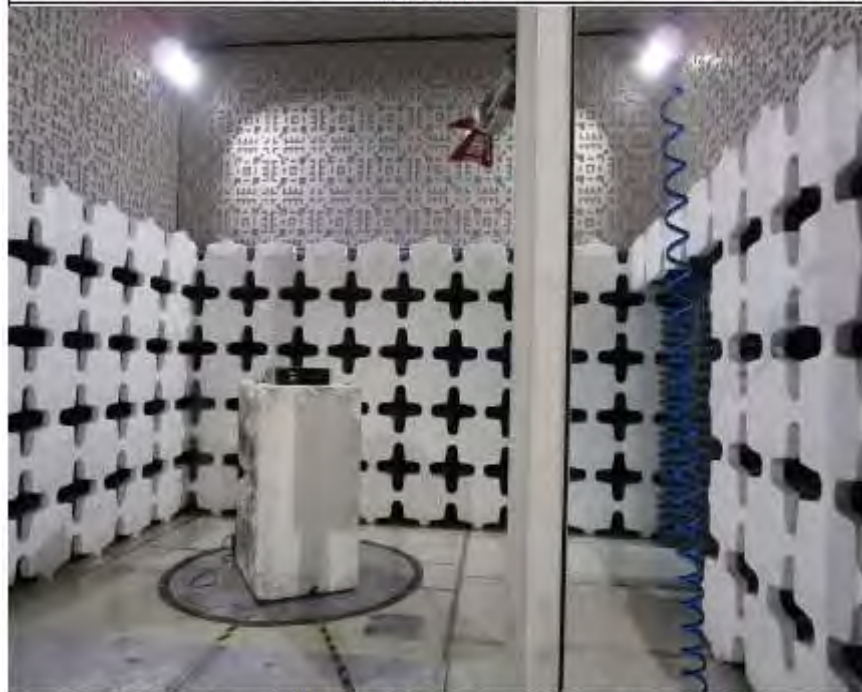
Test Setup for Spurious Radiated Emissions, Above 1GHz – Antenna Polarization Vertical
