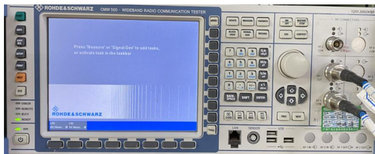
CMW 500 (2G/3G/4G Test Equipment)
