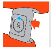
► Turn Romware ONE™ on by pushing the Multi-function button until the Light-ring indicator lights up blue. Let go of the button, the light ring indicator starts filling up blue while the device is starting.
