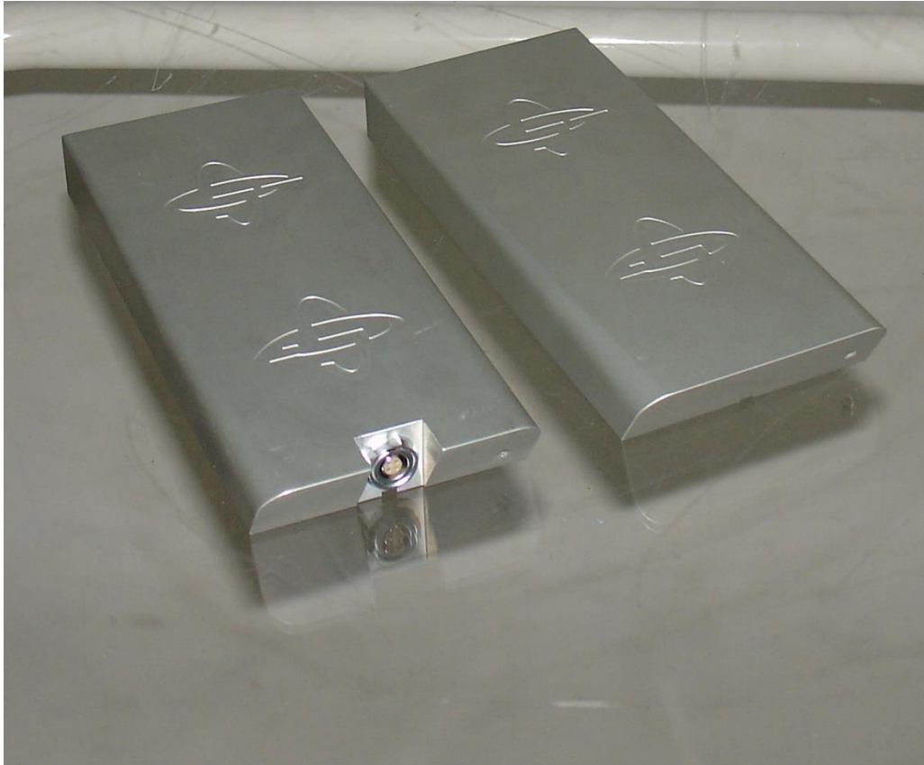
Batteries, left dummy battery-case with feed trough cable for central system battery operation, right; li-ion battery for transducer only.
