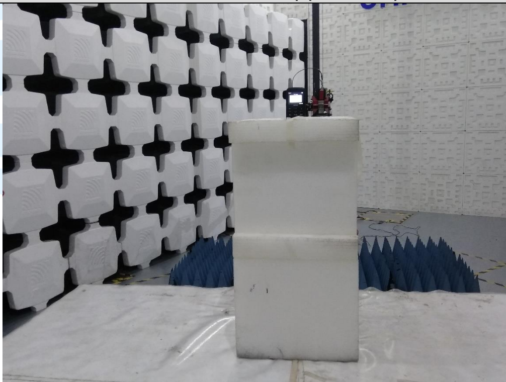
Radiated emission Test Setup (Above 1 GHz)
