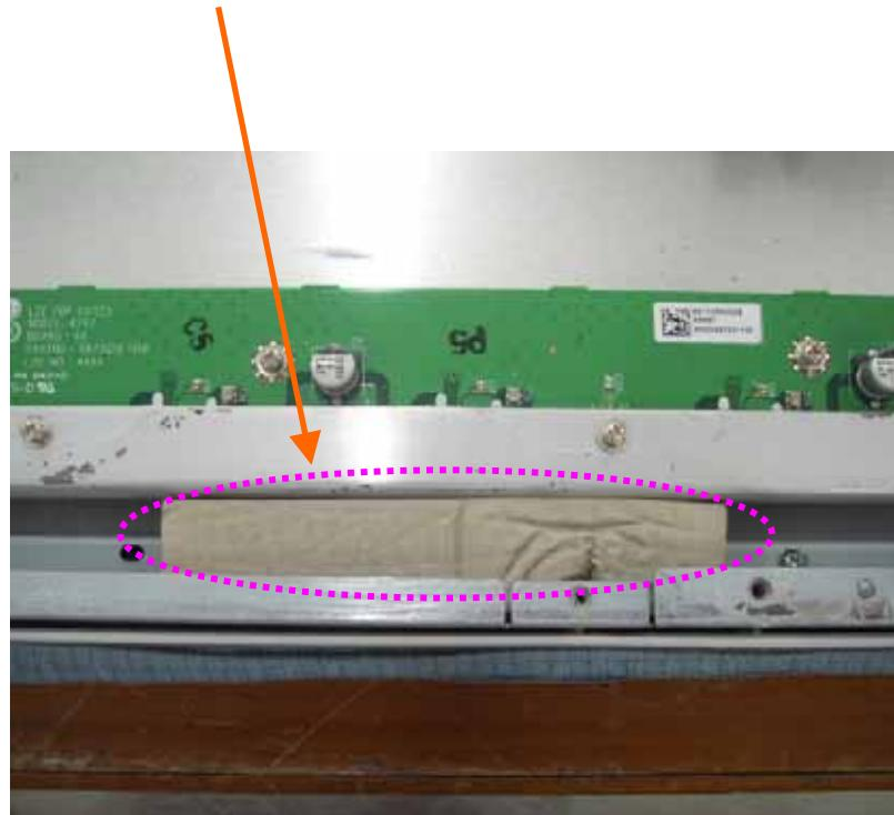
**2. Attach a gasket and a Core**
