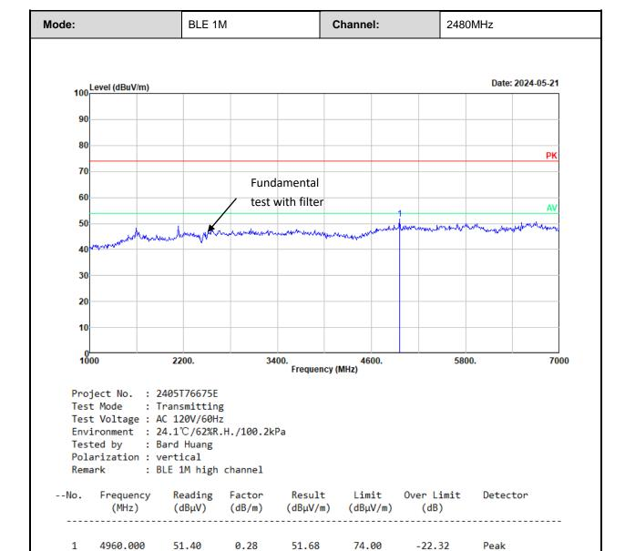
Remarks: Factor = Antenna factor + Cable loss - Preamp gain Result = Reading + Factor
