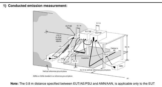
being measured. If the device is AE then it shall be >0.8 m.
