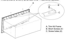
5. Release the 4 locating pins from locating holes, take out the trim kit frame, and set aside.
