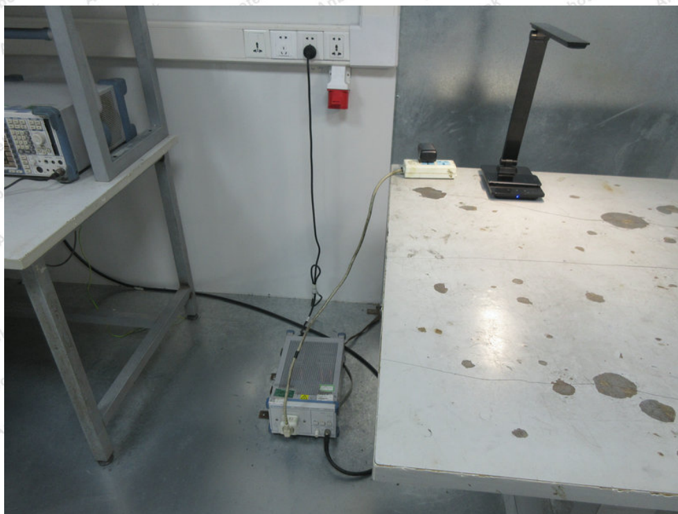
Photo of Conducted Emission Measurement
