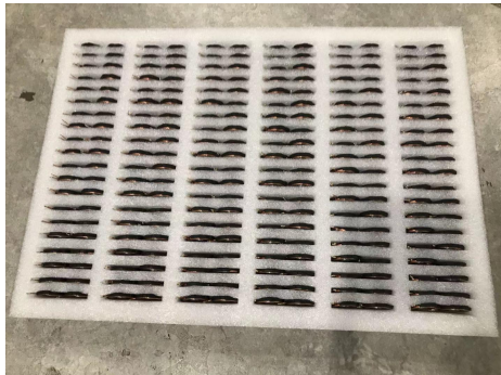
图 2：统一方向线头朝上整齐排放入盘中 Figure 2: Uniform Direction Line head up neatly into the disk
