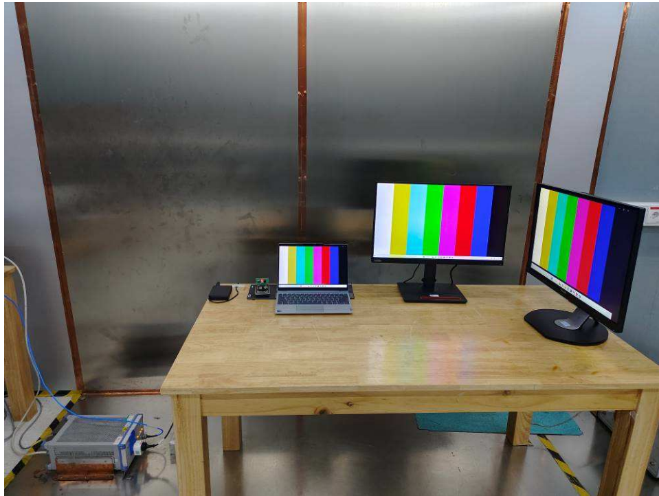
Photograph 1: Set-up for Conducted Emission on AC Mains
