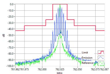
Analogue Modulation 762.0250MHz Mask B 1W RBW=300Hz, VBW=3000Hz, Detector Mode=Peak Result=Pass
