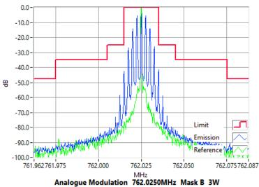
Analogue Modulation 762.0250MHz Mask B 3W RBW=300Hz, VBW=3000Hz, Detector Mode=Peak Result=Pass
