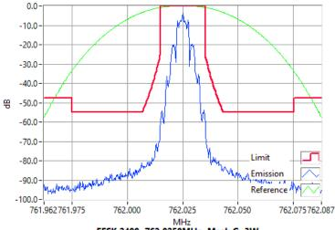
FFSK 2400 762.0250MHz Mask G 3W RBW=300Hz, VBW=3000Hz, Detector Mode=Peak Result=Pass
