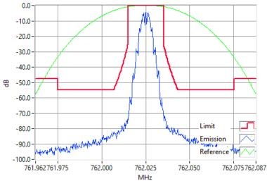
FFSK 1200 762.0250MHz Mask G 3W RBW=300Hz, VBW=3000Hz, Detector Mode=Peak Result=Pass
