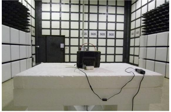
Radiated Emission Set up Photos (Below 1GHz)
