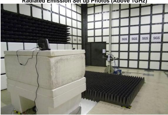
Radiated Emission Set up Photos (Above 1GHz)
