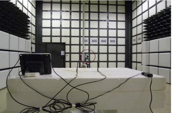
Radiated Emission Set up Photos (Below 1GHz)
