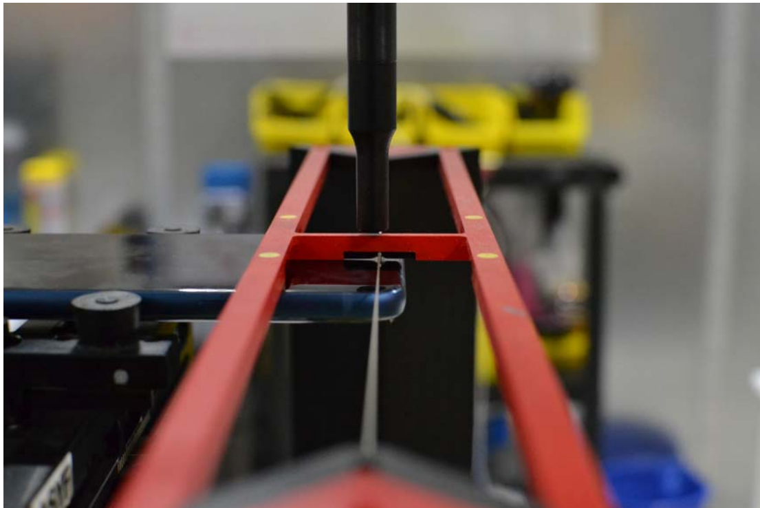
Figure 18-2 HAC Phantom Plane Alignment
