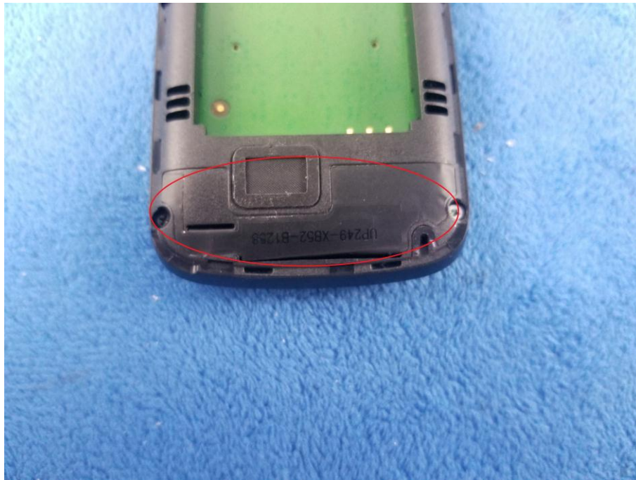
GSM/PCS/UMTS-FDD Antenna View
