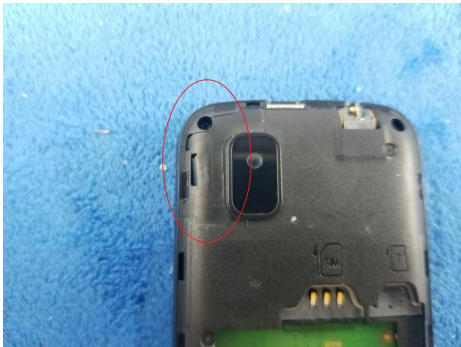
WIFI/BT/BLE/GPS - Antenna View
