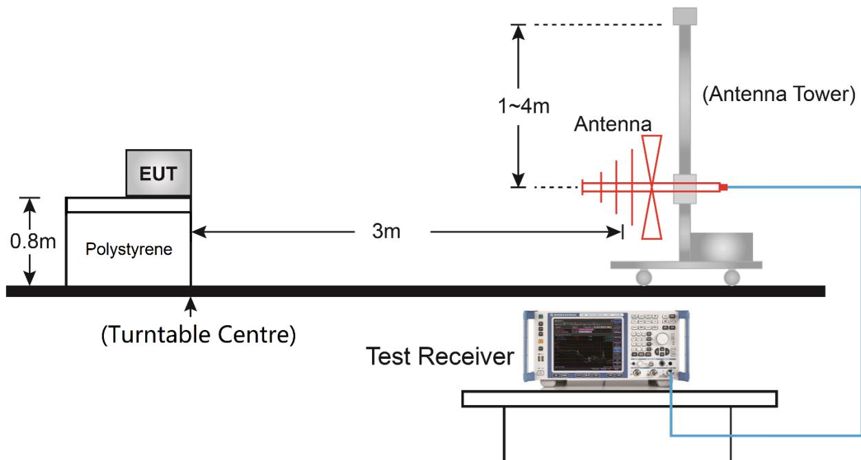
Above 1GHz Test Setup:
