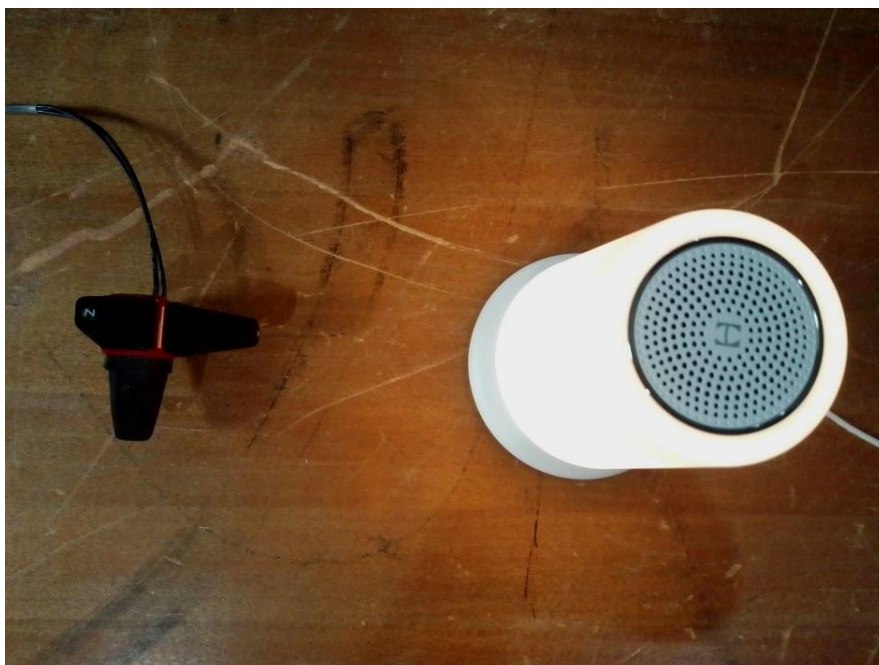
E-Field Strength View Position A (Distance 15cm)
