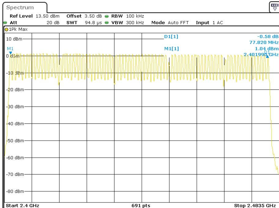
**EDR ( $\pi/4$ -DQPSK): Number of Hopping Channels**
