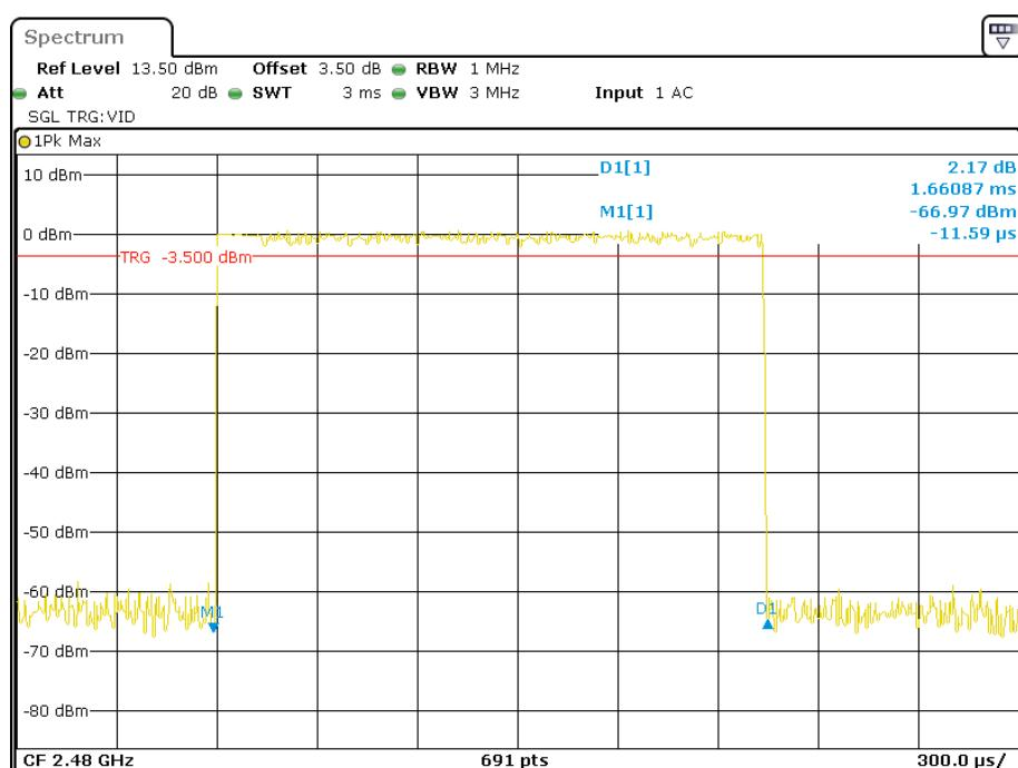
**Pulse time, Low Channel, 3DH5**
