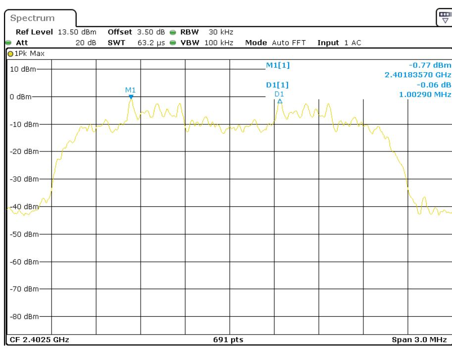
**EDR ( $\pi/4$ -DQPSK): Middle Channel**
