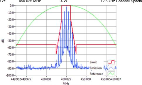
Analogue Modulation 450.0250MHz Mask D 4W RBW=100Hz, VBW=1000Hz, Detector Mode=Peak Result=Pass
