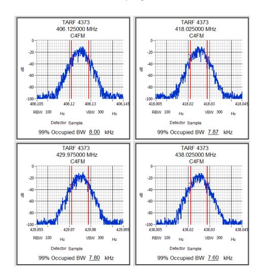
Channel 5-7 4 watts 12.5 kHz ch spacing P25 Phase 1 C4FM Modulation
