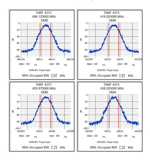
Channel 5-7 4 watts 12.5 kHz ch spacing DMR Modulation
