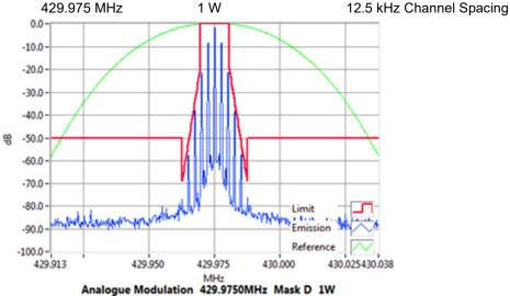
Analogue Modulation 429.9750MHz Mask D 1W RBW=100Hz, VBW=1000Hz, Detector Mode=Peak Result=Pass
