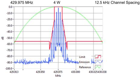
Analogue Modulation 429.9750MHz Mask D 4W RBW=100Hz, VBW=1000Hz, Detector Mode=Peak Result=Pass
