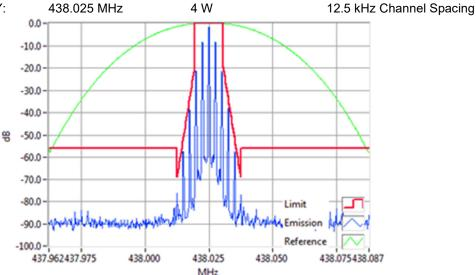
Analogue Modulation 438.0250MHz Mask D 4W RBW=100Hz, VBW=1000Hz, Detector Mode=Peak Result=Pass
