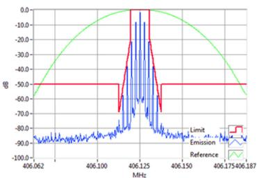
Analogue Modulation 406.1250MHz Mask D 1W RBW=100Hz, VBW=1000Hz, Detector Mode=Peak Result=Pass
