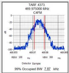
Channel 1-4 4 watts 12.5 kHz ch spacing P25 Phase 2 HCPM Modulation
