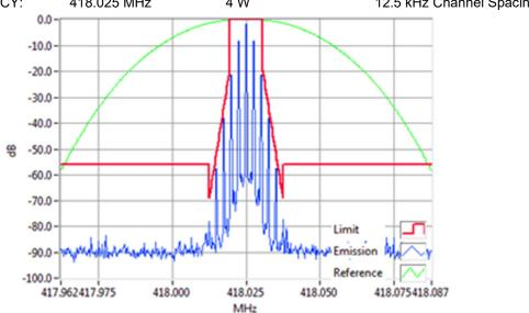
Analogue Modulation 418.0250MHz Mask D 4W RBW=100Hz, VBW=1000Hz, Detector Mode=Peak Result=Pass
