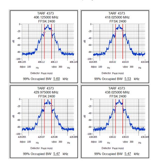
Channel 5-7 4 watts 12.5 kHz ch spacing FFSK 2400 Modulation
