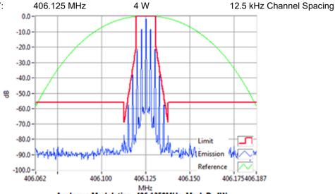
Analogue Modulation 406.1250MHz Mask D 4W RBW=100Hz, VBW=1000Hz, Detector Mode=Peak Result=Pass
