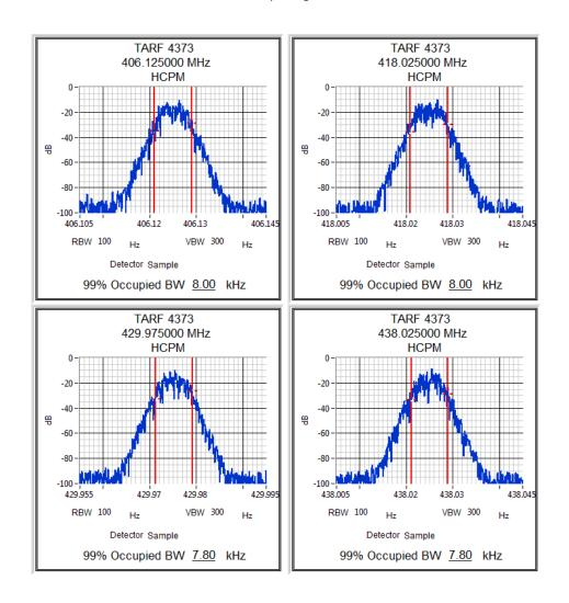
Channel 5-7 4 watts 12.5 kHz ch spacing P25 Phase 2 HCPM Modulation
