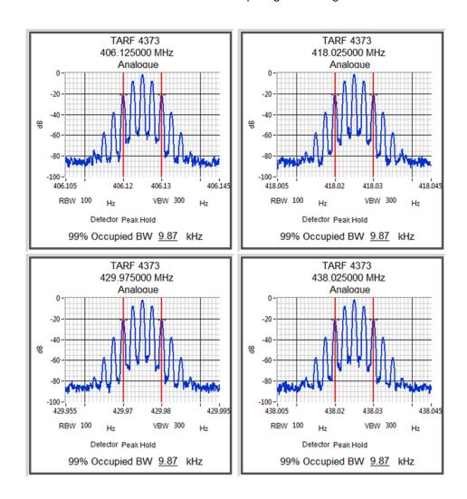
Channel 5-7 4 watts 12.5 kHz ch spacing Analogue Modulation
