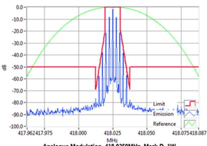
Analogue Modulation 418.0250MHz Mask D 1W RBW=100Hz, VBW=1000Hz, Detector Mode=Peak Result=Pass
