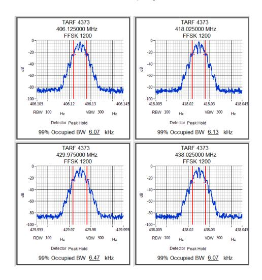
Channel 5-7 4 watts 12.5 kHz ch spacing FFSK 1200 Modulation
