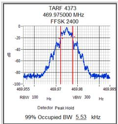
Channel 1-4 4 watts 12.5 kHz ch spacing DMR Modulation
