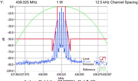
Analogue Modulation 438.0250MHz Mask D 1W RBW=100Hz, VBW=1000Hz, Detector Mode=Peak Result=Pass
