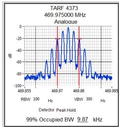
Channel 1-4 4 watts 12.5 kHz ch spacing FFSK 1200 Modulation
