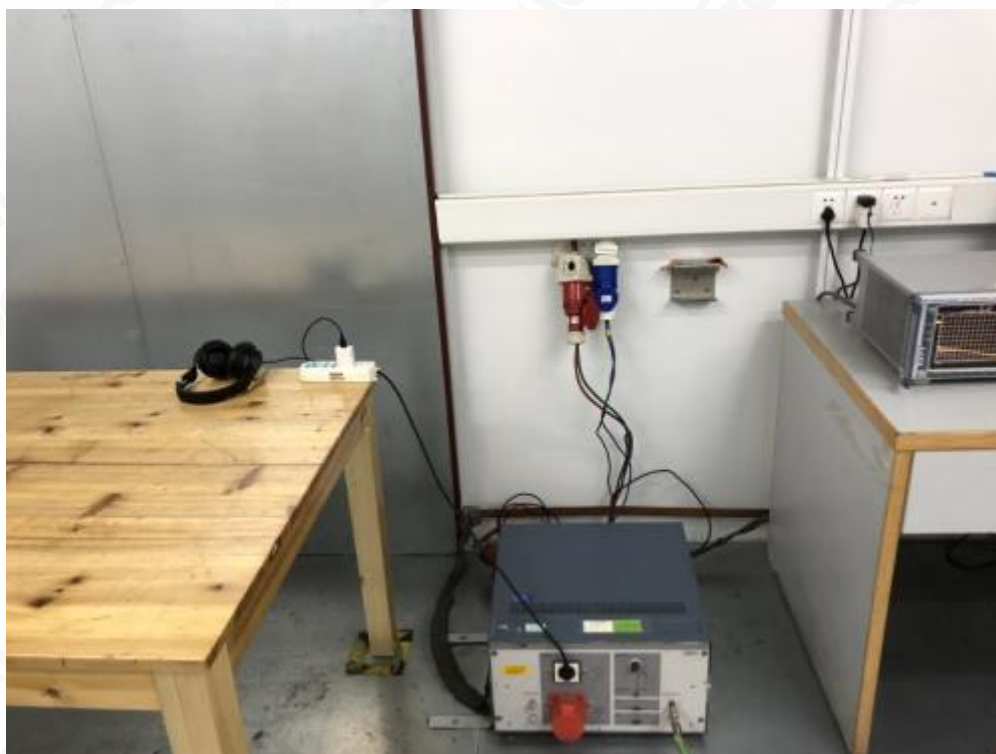
RADIATED EMISSION TEST SETUP BELOW 1GHz
