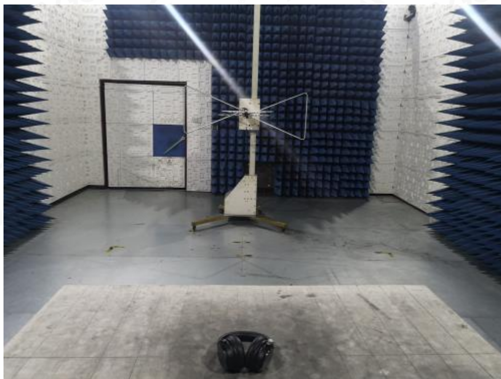
RADIATED EMISSION TEST SETUP BELOW 1GHz
