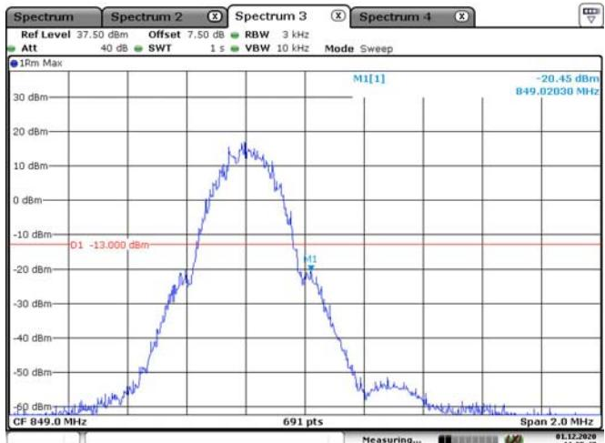
**GSM 1900, Left Band Edge**
