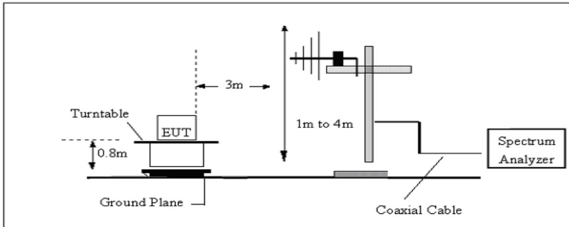
(B) Radiated Emission Test-Up Frequency Above 1GHz
