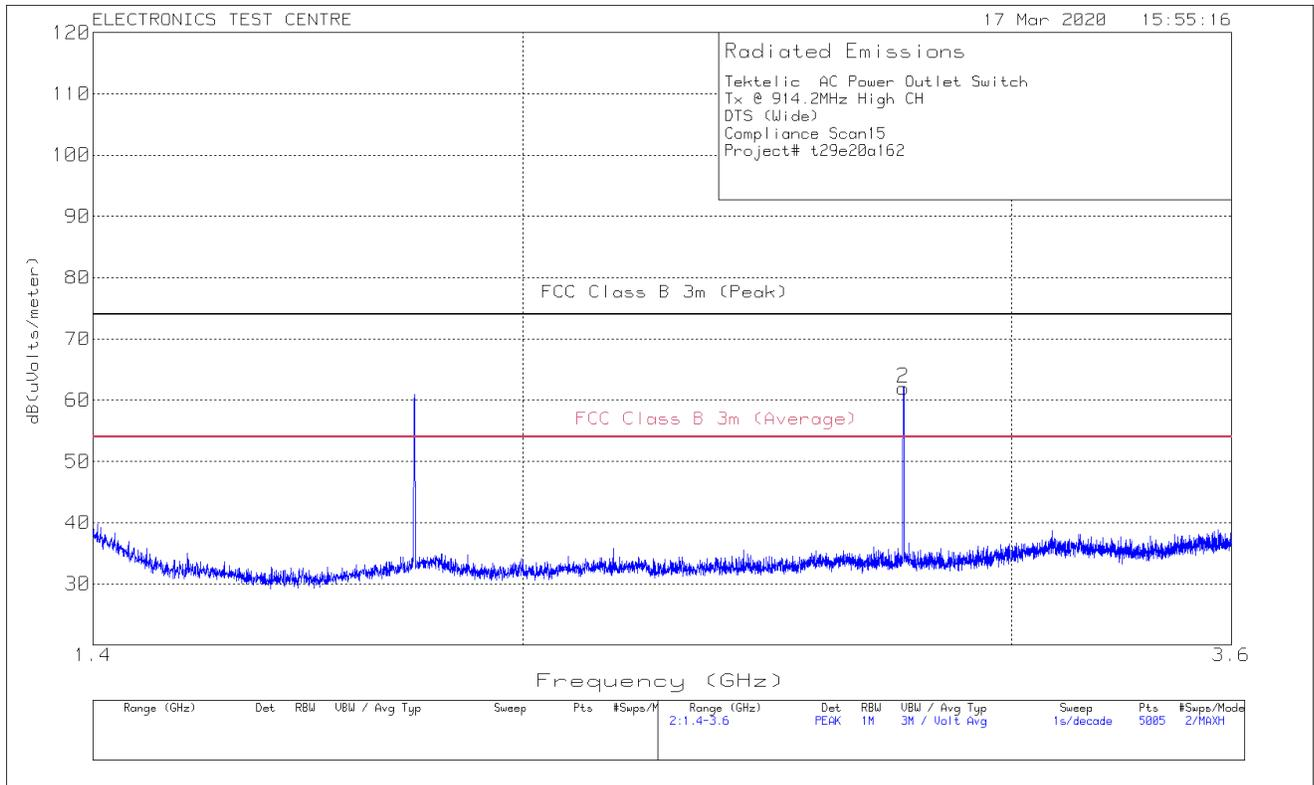
**Plot of Radiated Emissions: Horizontal polarization**
