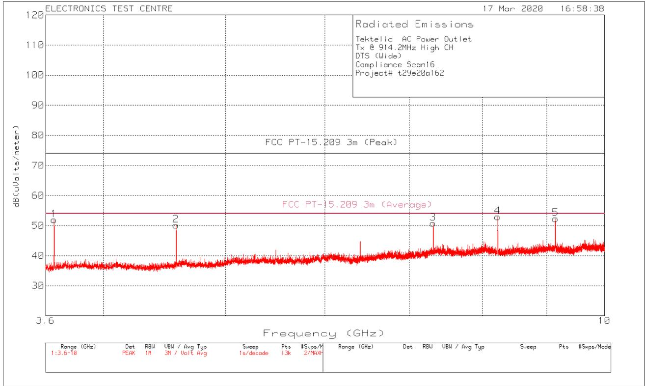
**Plot of Radiated Emissions: Vertical polarization**
