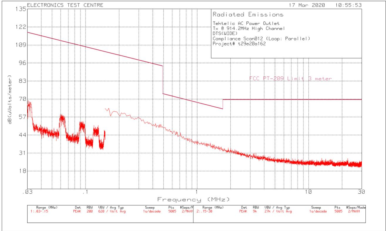
**Plot of Radiated Emissions: Measuring Antenna Perpendicular**
