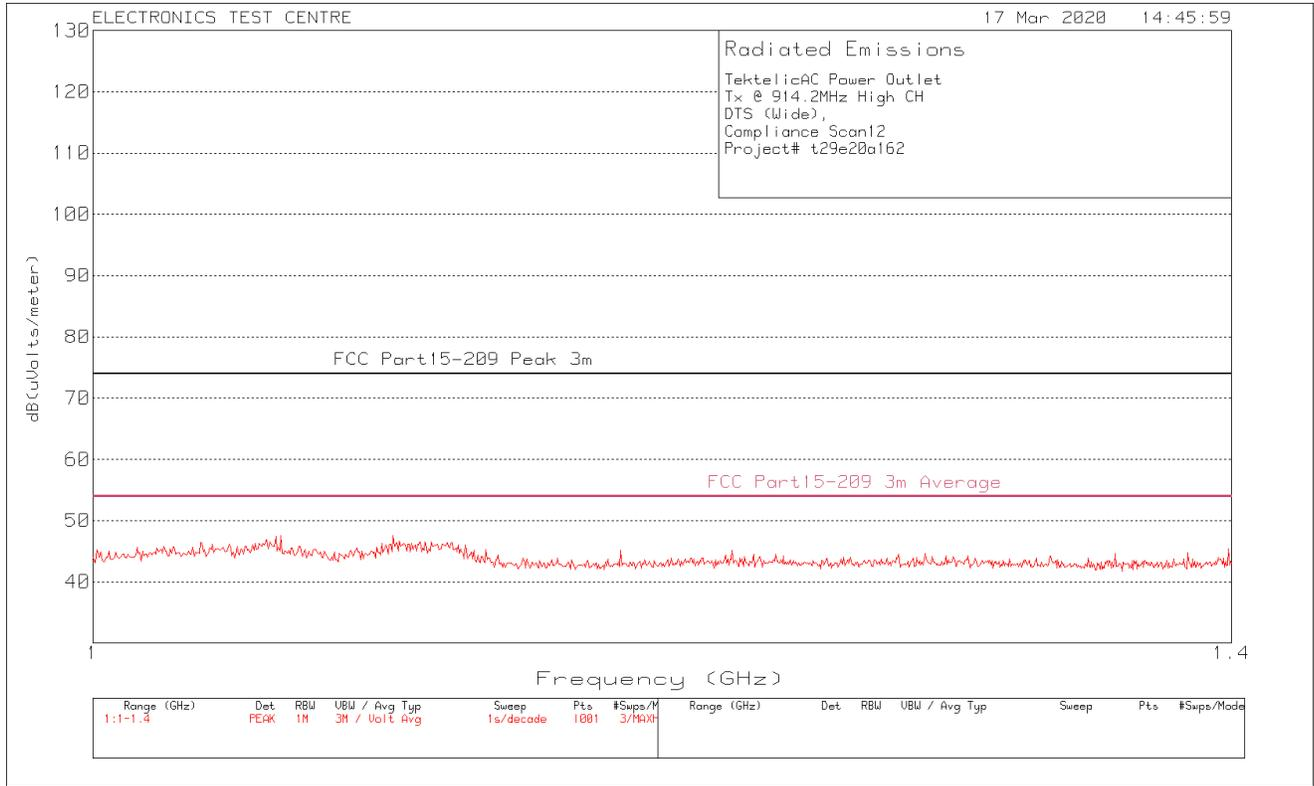
**Plot of Radiated Emissions: Vertical polarization**
