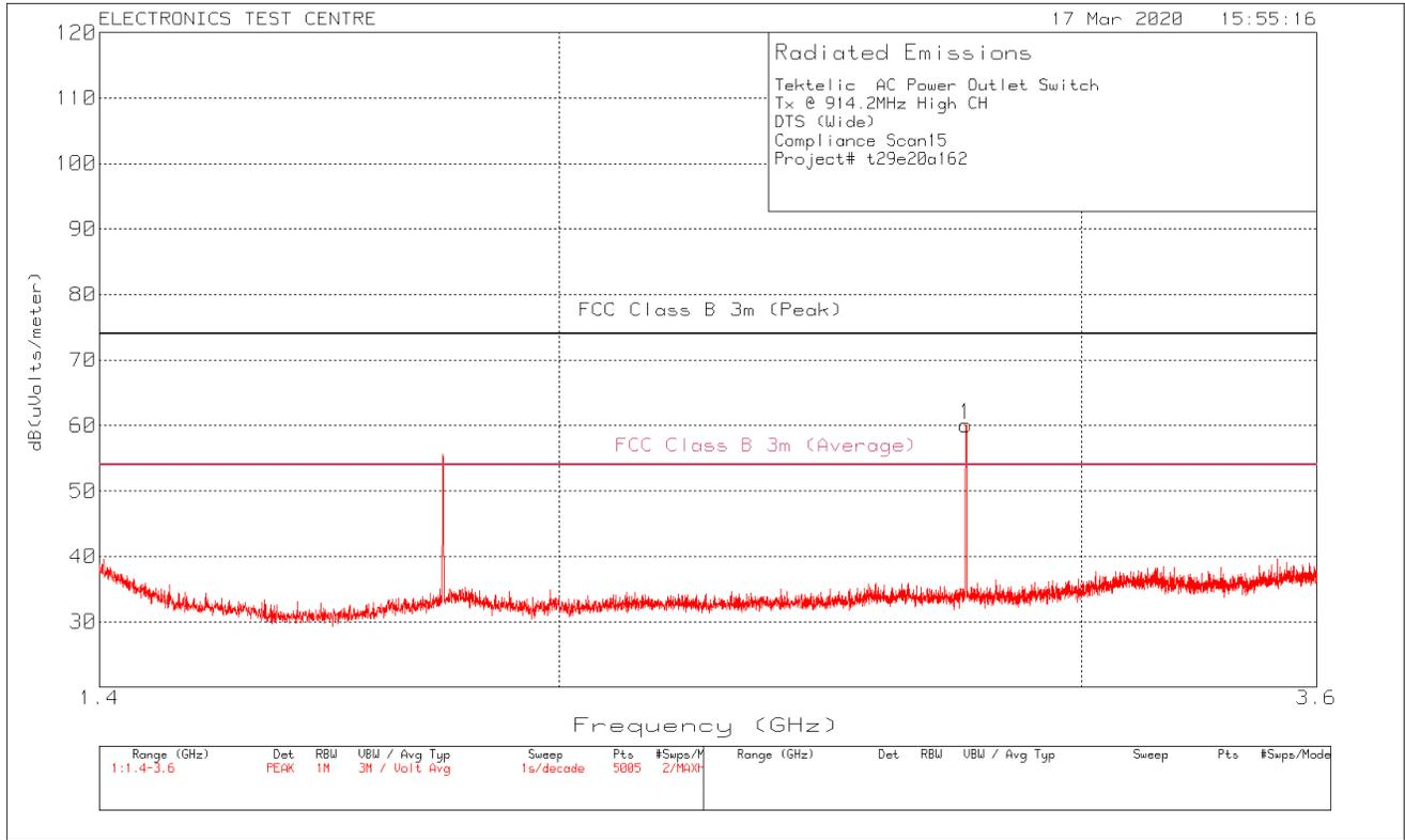
**Plot of Radiated Emissions: Vertical polarization**
