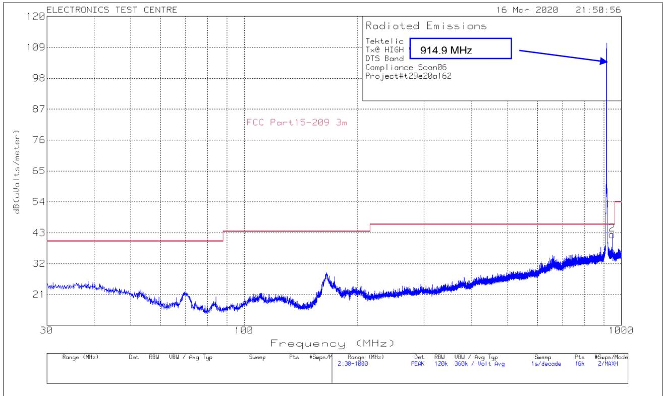
**Plot of Radiated Emissions: Horizontal polarization**
