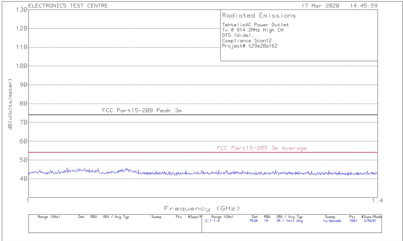
**Plot of Radiated Emissions: Horizontal polarization**
