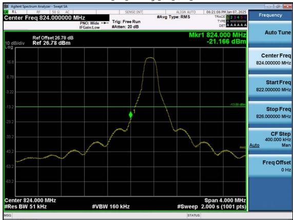
LTE B5\_5 M\_Band Edge\_Low\_QPSK\_1RB
