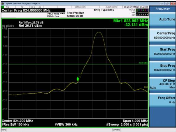
LTE B5\_10 M\_Band Edge\_Low\_QPSK\_1RB
