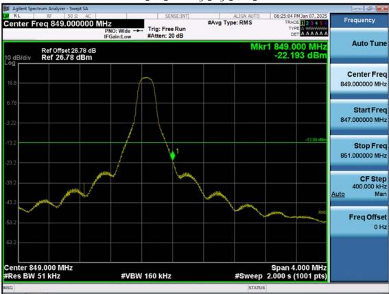
LTE B5\_5 M\_Band Edge\_High\_QPSK\_1RB
