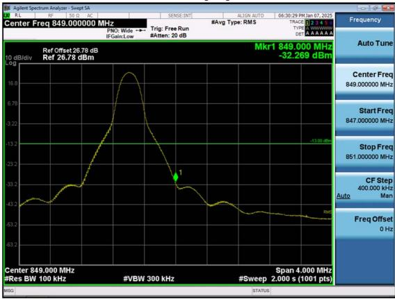
LTE B5\_10 M\_Band Edge\_High\_QPSK\_1RB
