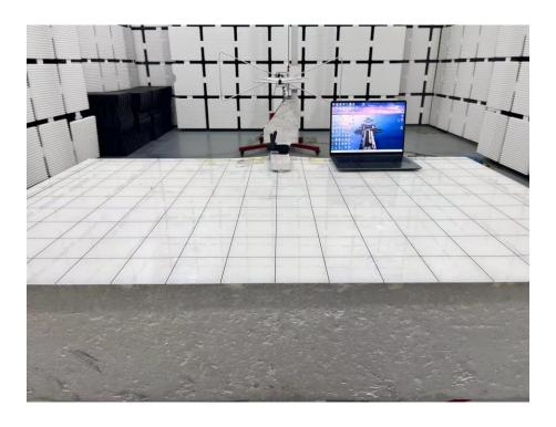
Set-up for Radiated Spurious Emission, Above 1GHz
