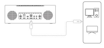
2. Press Mode Switch/Mute Button and switch to optical input. Notice tone "Optical Input" will be heard.
