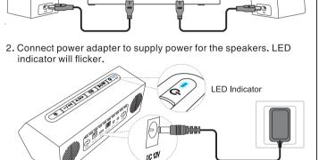
3. Long press and hold Power On/Off Button for 3 seconds to turn on the speakers. LED indicator will change to be always on and RGB of satellite speakers will be on.
