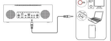
2. Press Mode Switch/Mute Button and switch to auxiliary input. Notice tone "Auxiliary Input" will be heard.
