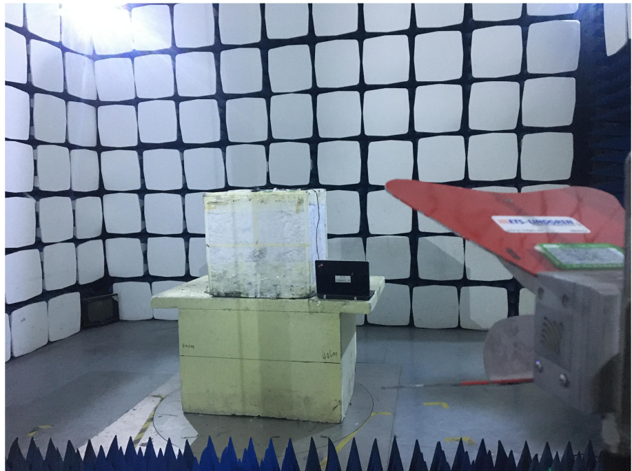
Radiation Emission Test Setup (1GHz to 18GHz)
