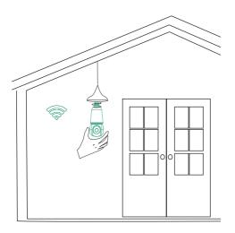
Please install the camera face down as shown in the picture. Wrong installation method may lead to product leakage and rapiddamage
