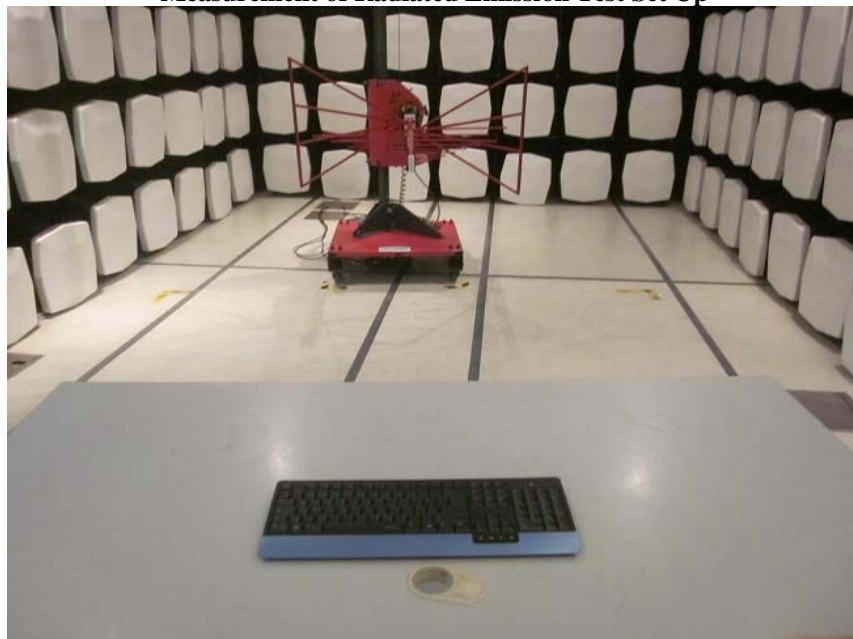
Measurement of Radiated Emission Test Set Up
