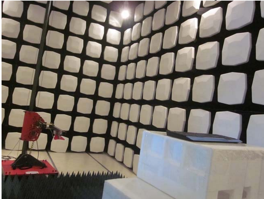
Measurement of Radiated Emission Test Set Up
