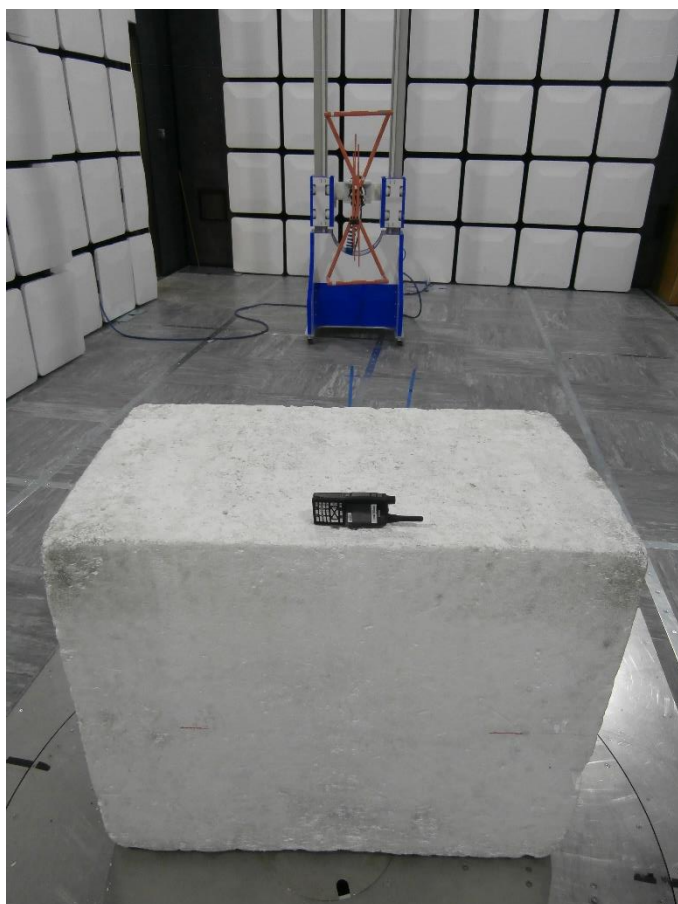
Figure 16 - Test Setup - 30 MHz to 1 GHz - Z Orientation
