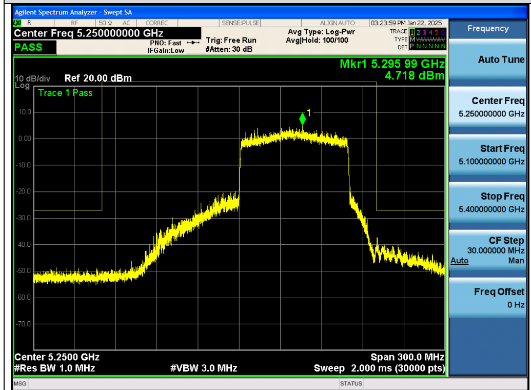
Test_Graph_802.11ax80_Chain A_5290_MCS0_Frequency Band 3
