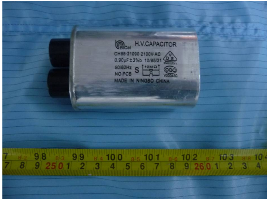
EUT – H.V. Capacitor View
