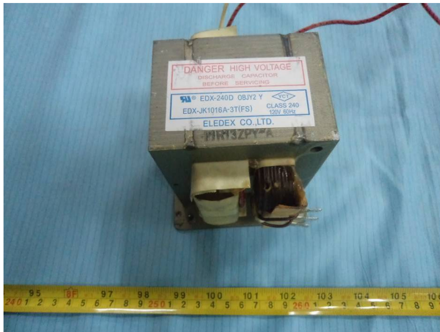
EUT – Power Transformer View
