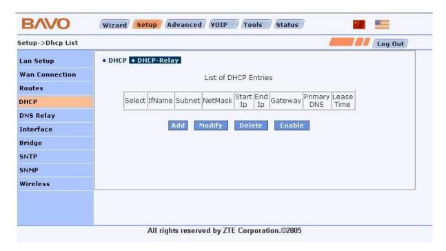
In the **DHCP Server Configuration Interface**, you can set the configurations of the DHCP server.
