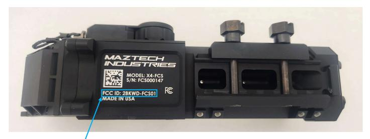
Label containing FCC ID & IC ID laser-etched into bottom surface
