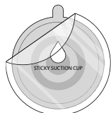
2. Peel off the protective film on the Suction Cup and press mount firmly onto the dashboard pad.
