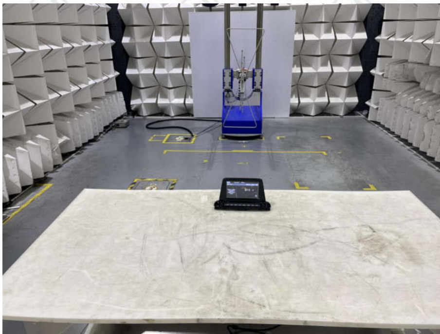
Radiated spurious emission Test Setup-1(Below 1GHz)
