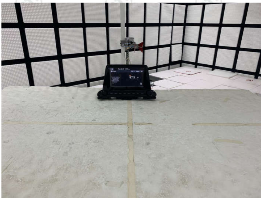
Radiated spurious emission Test Setup-2(Above 1GHz)
