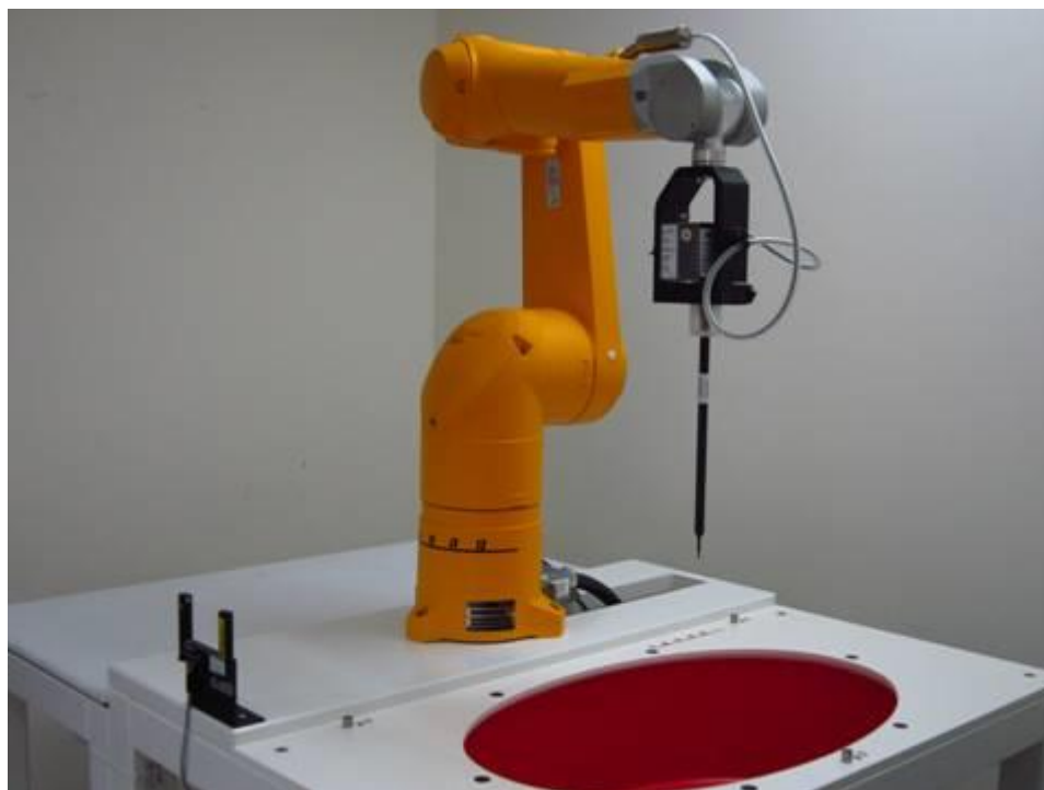
Fig.1 Photograph of the SAR measurement system
