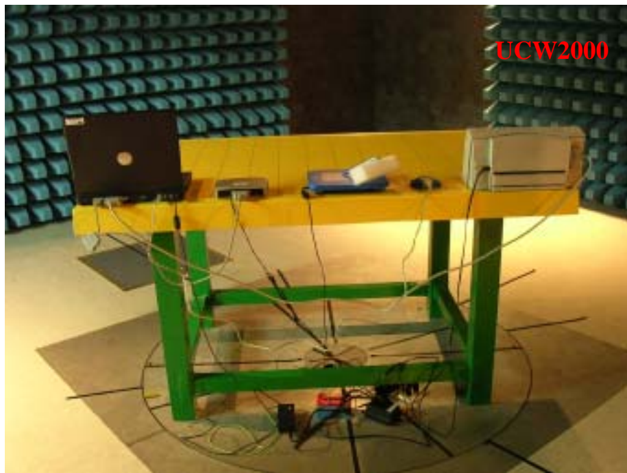
Photo 2: Radiated Emission Test Set-up
