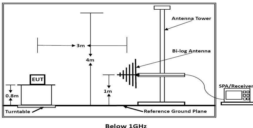
The radiated emission tests were performed in the 3 meters chamber test site, using the setup accordance with the ANSI C63.10-2013. The specification used was the FCC 15.209 and FCC 15.205 limits.
