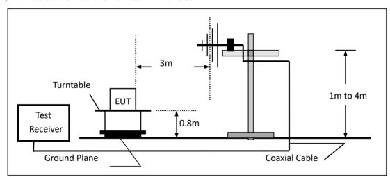
(c) For radiated emissions above 1000MHz
