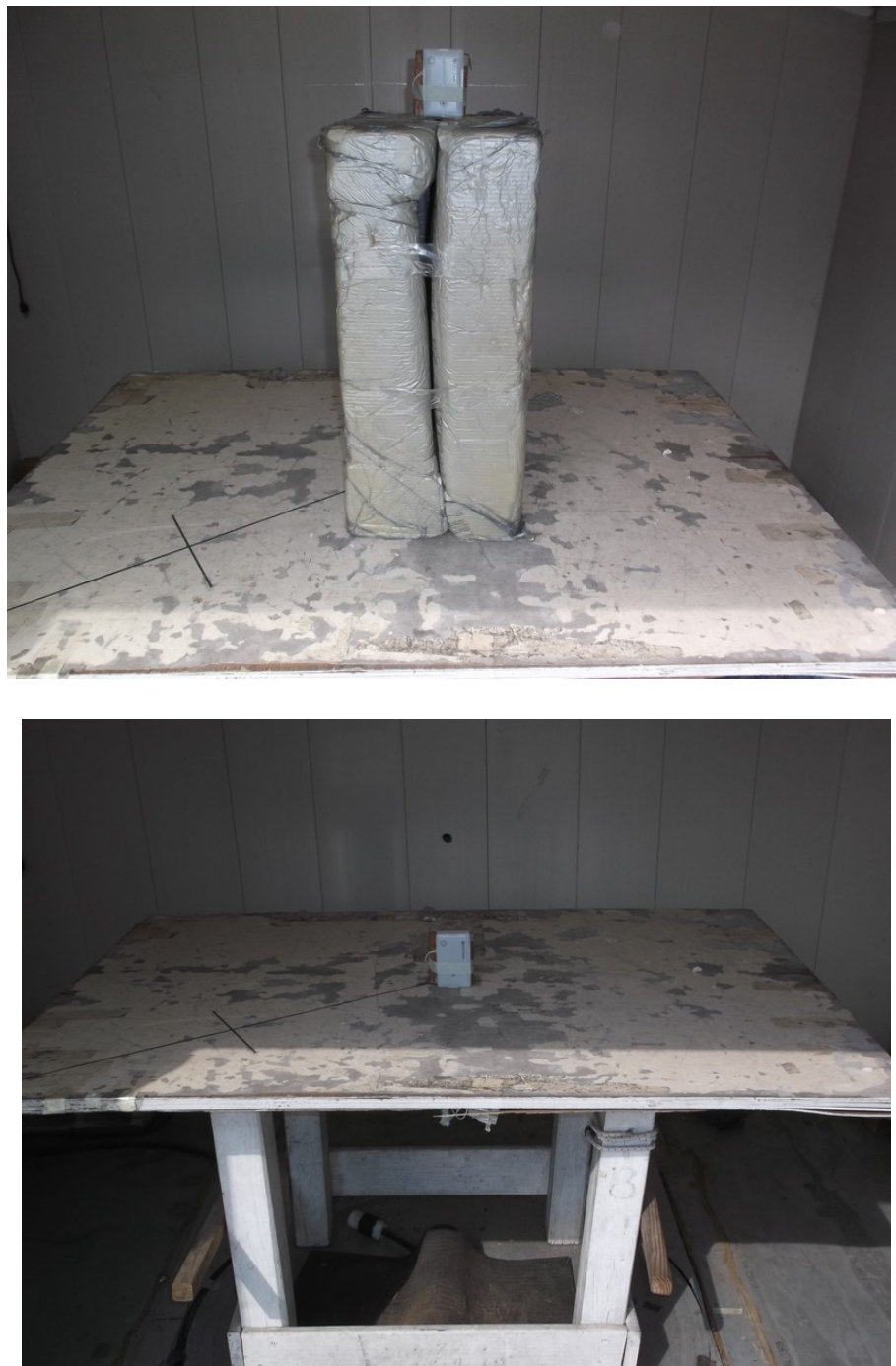
Figure 1 EUT Configuration for Radiated Emission Tests
