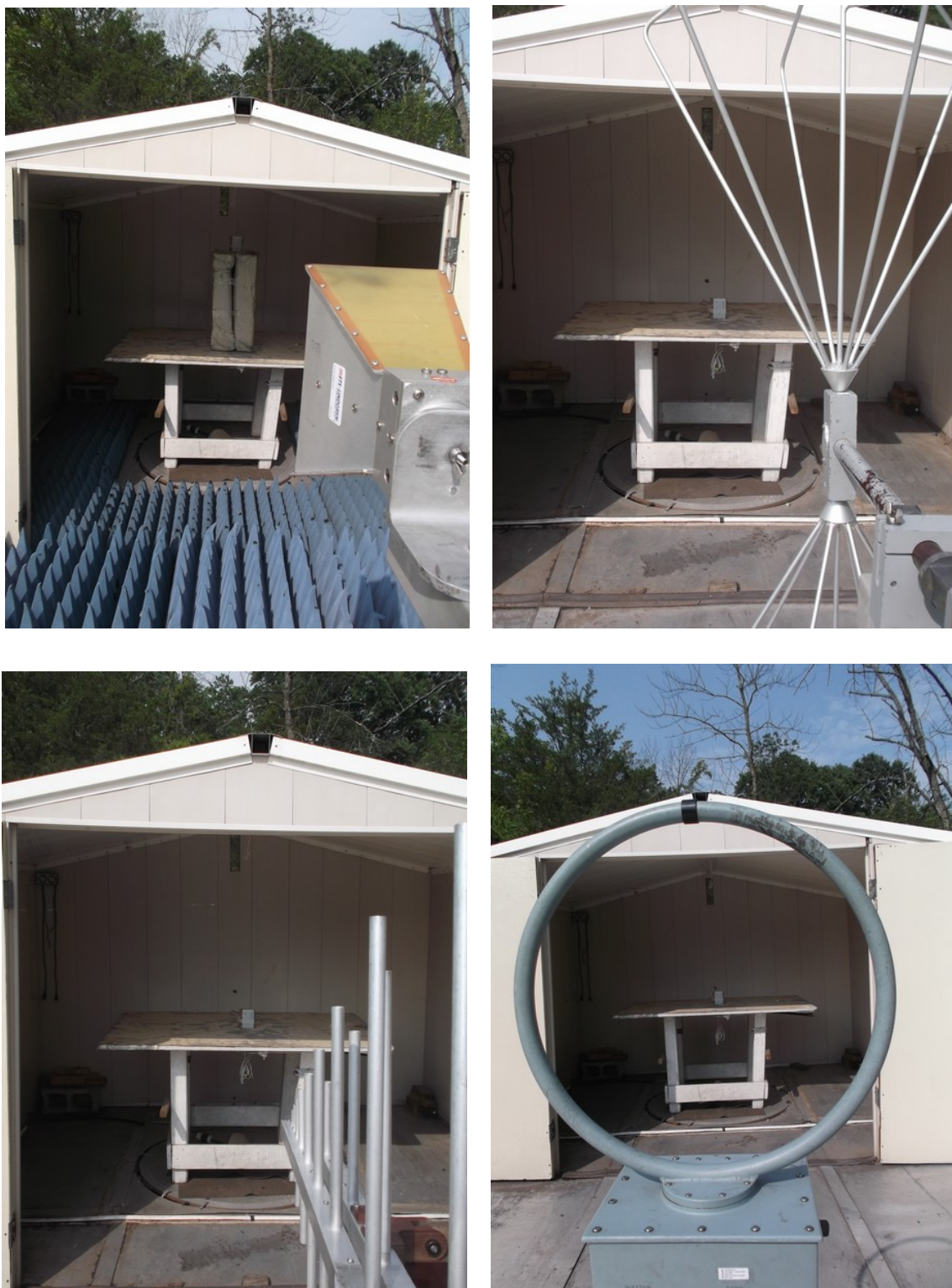
Figure 2 Radiated Emission Test Setup
