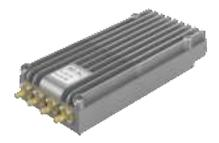
The E62-AU-AC – Active Combiner Module is the interface to the operator base station signal source equipment. Each module has four QMA ports for signal input from the maximum four operators. One Access Unit can be equipped with up to four modules. In accordance with wireless service provider standards, it is not advised to use digital repeaters as a signal source for Corning solutions.
