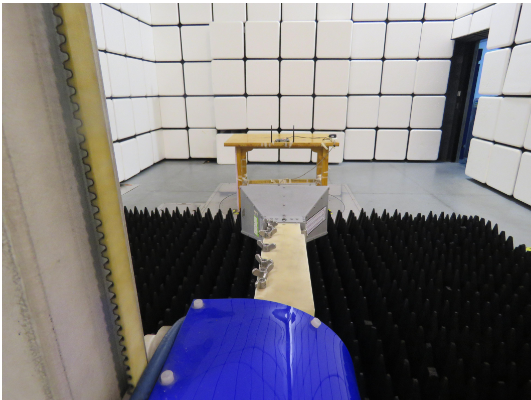
Picture 2: Radiated Spurious Emissions Test setup
