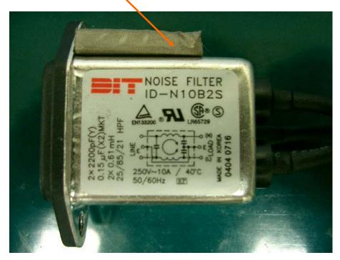
4. Attach a gasket on PDP Panel and Main Frame
