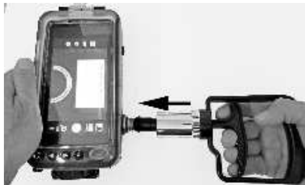
Hand pump pressed against vacuum check port
