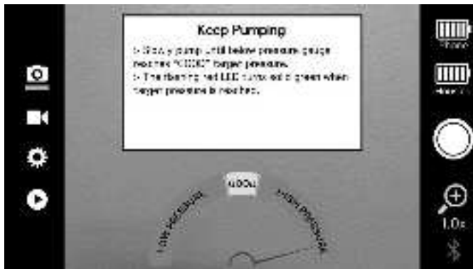
Pump until gauge needle reaches “GOOD”
