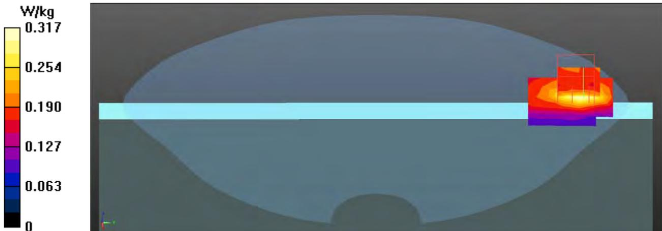
**802.11ac (80M) EUT Back(PAD) (SPEED Aux Antenna), Z-Axis plot**
