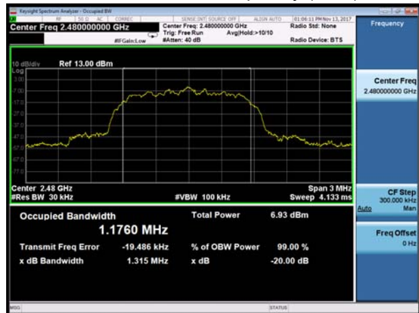
BT 2DH5 CH78, Carrier frequency (MHz): 2480
