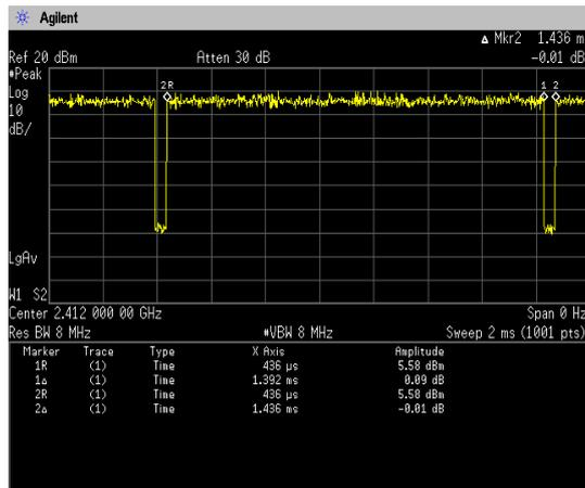
$$\text{Duty Cycle} = \text{Ton} / (\text{Ton} + \text{Toff}) = 1392[\mu\text{s}] / (1392[\mu\text{s}] + 44[\mu\text{s}]) = 96.94[\%]$$
