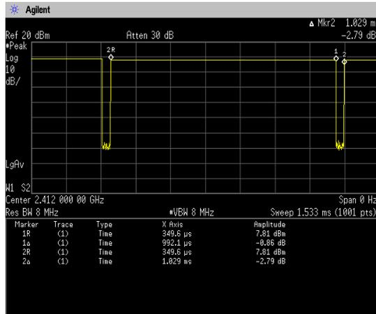
$$\text{Duty Cycle} = \text{Ton} / (\text{Ton} + \text{Toff}) = 992.1[\mu\text{s}] / (992.1[\mu\text{s}] + 36.9[\mu\text{s}]) = 96.41[\%]$$
