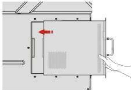
Step 3: Ensure that the distance between the rear pluggable computer and the installation wall for heat dissipation is not less than 20.0mm (as shown in the figure below, taking installation on a large screen as an example).
