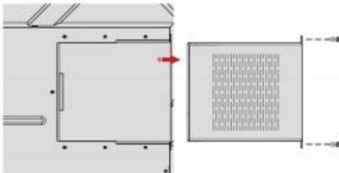
Step 2: Push the pluggable computer horizontally into the dedicated interface card slot as shown in the diagram.
